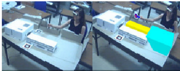
Figure 44: User modelling with tangible interfaces (paddles) overlaying virtual objects onto a physical model. On left visualising in Reality and on the right visualised in Augmented Reality [Dias, 2002]
